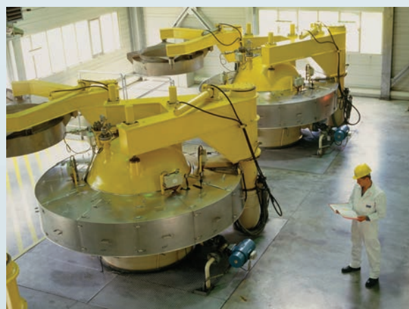
Industrial autoclaves using scCO 2 in a food processing plant.
