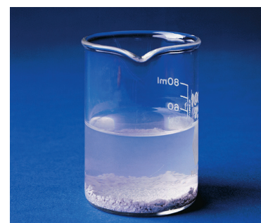
▲ \text{AgCl} does not significantly dissolve in water; it remains as a white powder at the bottom of the beaker.
